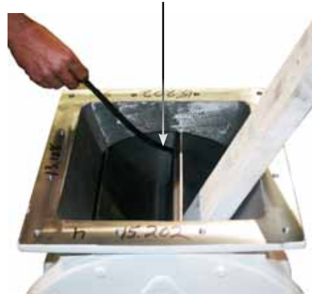
Use Feeler Gauge to Check Clearance Between Rotor and Endplate
