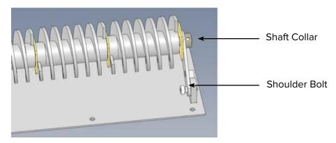
Figure 6 Bolt and Shaft Locations
