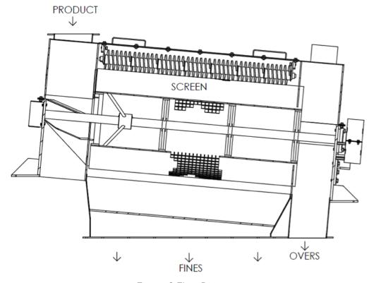
Figure 3 Flow Diagram
