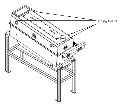
Figure 2 Lifting Points
