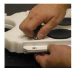
Insert fasteners along the length of the support frame and tighten to recommended torque values.
