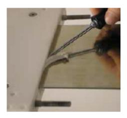
Using shears or scissors cut one end of the new packing cord at a 45° angle.
