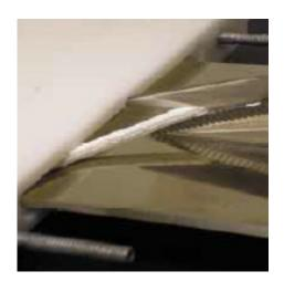
Repeat steps 7 through 9 for the second packing cord. When installing the second packing cord place the seam on the opposite side of the blade as the first packing cord seam.
