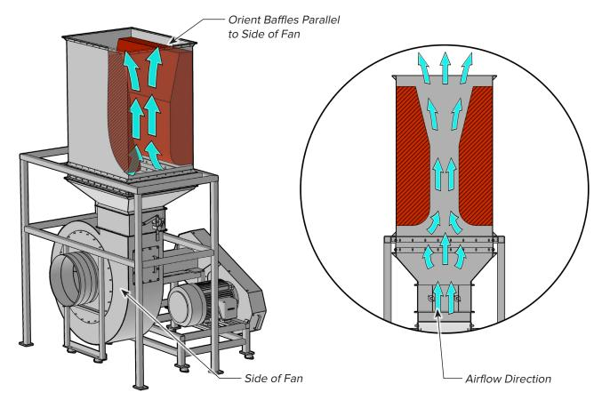
When installing the fan silencer it is important to note the direction of the air flow and orientation of the acoustic baffles relative to the fan housing. The air should flow through the smooth, rounded end of the baffles and out the wider, angled end of the baffle. The baffles should also be oriented to be parallel with the sides of the fan housing.
